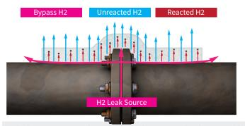
As hydrogen gas passes through the membrane, H2 molecules react with colorimetric pigment, accumulating over time and changing the tape from translucent gray to black indicating a leak is present.
